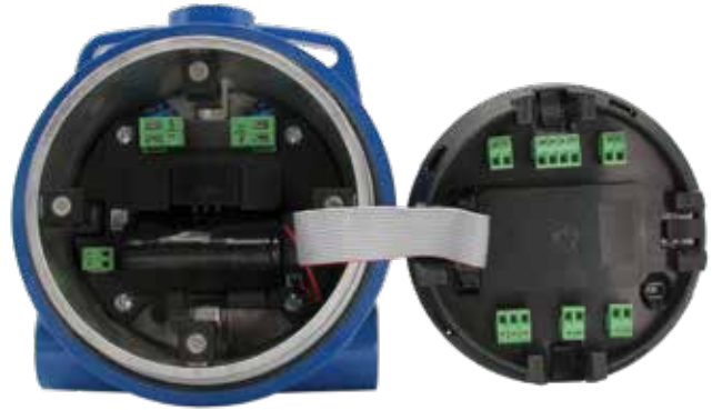
Options Module (Left) and Display Module (Right)
